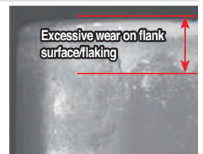
Existing grade (K15)
