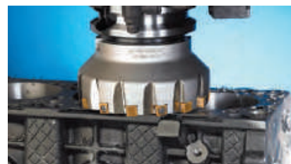
Roughing for cast iron
