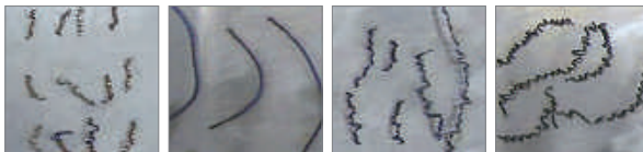
VL Chip Breakers Competitor A Competitor B Competitor C
