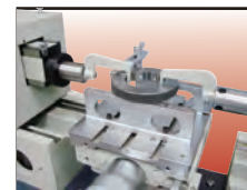
Small size ring gauge calibration with inner double yoke
