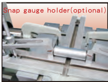
External snap gauge calibration
