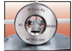
Inner thread gauge measurement
