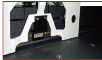
XYZ axis reflection type metal grating measurement system
