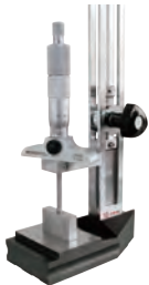
■ Depth micrometer calibration
