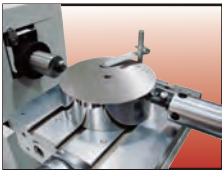
Cylinder gauge calibration
