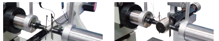
Optional accessories 3 wire thread gauge(for External thread measurement)
