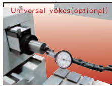
Level-type indicator calibration
