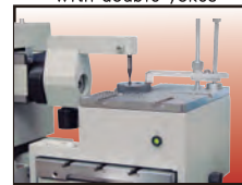
Small size ring gauge calibration with magic eye device
