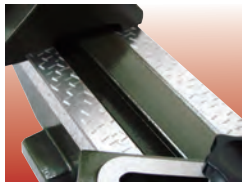
Precision grinding and scraping
