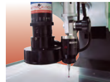
Zoom magnification optical lens and 3D touch probe
