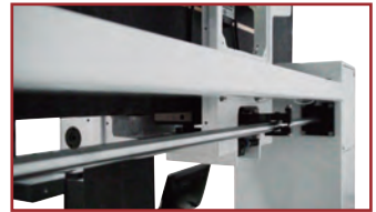
XYZ axis non-screw drive bar device for fine position adjustment
