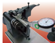
Example of measuring concentricity with indicator
