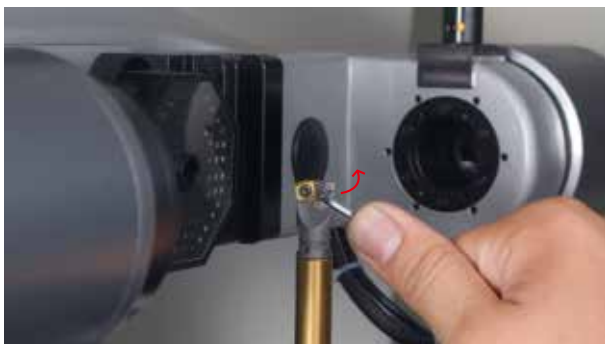
Direction to increase boring diameter.
