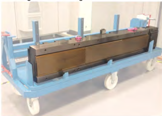
Steering rack broach holder and broach
