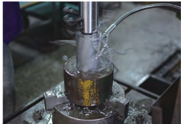
Operation of core drills on the drilling machine
