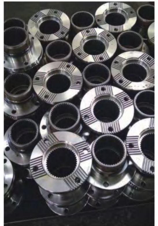
Sparts broaching by flat spline broach
