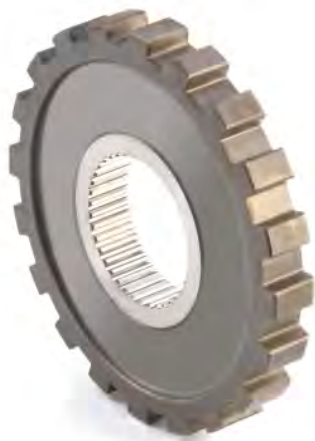
Part broached by carbide hard broach tools
