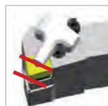
Optimal position and distance of spraying
