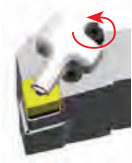
Unscrew the clamping screw
