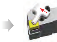
Move the water clamp to the edge of the holderscrew
