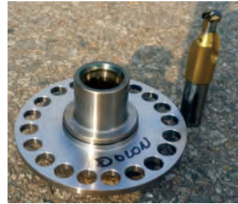
After drilling & back chamfering
