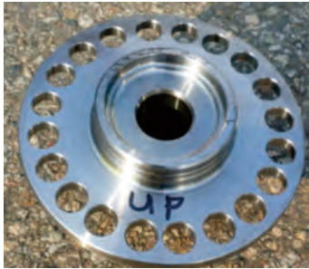
After drilling & front chamfering
